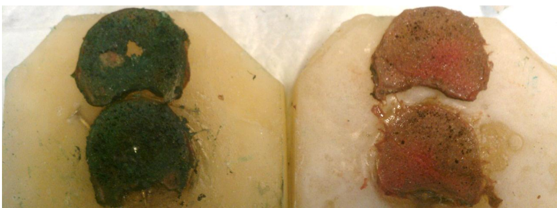
Figure 3.5 Results from second preliminary test. Note the blue-green color of the cancellous bone on the left. L1 shown on the left and T12 shown on the right. The difference in color is brought on by leaking of stain from the intervertebral disc, through the endplate fracture, and into the cancellous bone of the vertebra.
